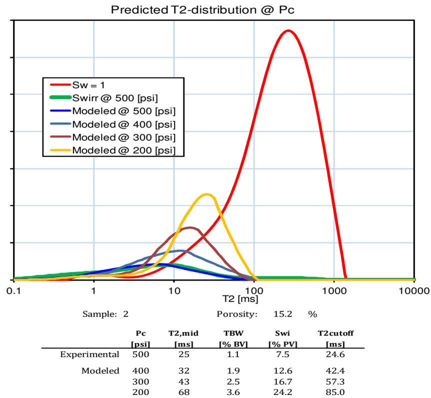
Figure 5 Predicted T2-distribution at experimental conditions and other [Hg-air] pressures for sample 2
